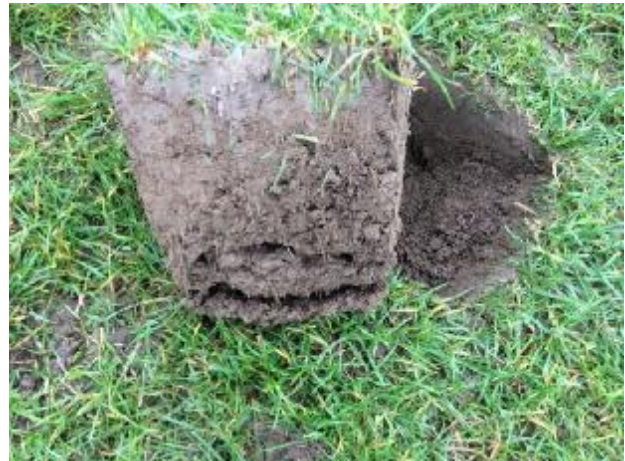
Figure 10: The pitch centres were more compact as shown above with a smeared layer. There was no evidence of sand dressings or secondary drainage installation.
